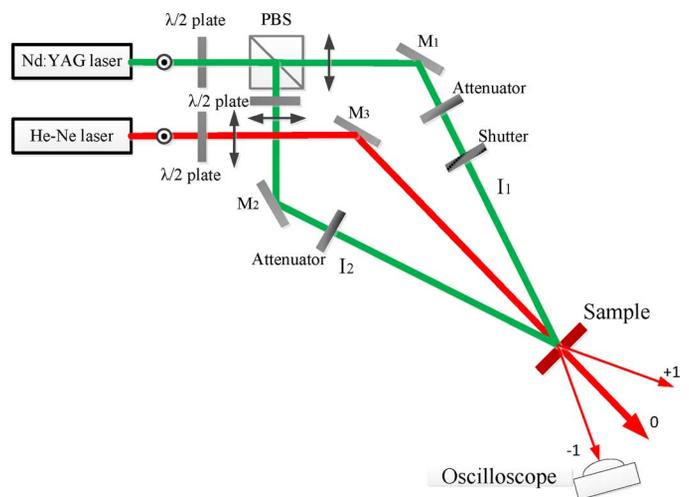
Fig. 3. Experimental setup for response time testing. M1–M3 are mirrors, BS is a beam splitter,  $\lambda/2$  is a half-wave plate.
