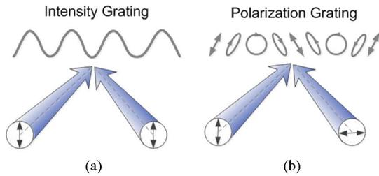
Fig. 7. Schematic illustrations of: (a) an intensity holographic exposure using parallel polarizations and (b) a polarization holographic exposure using crossed polarizations.
