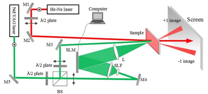
Fig. 9. Experimental setup for holographic video display.
