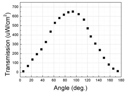
Fig. 2. Transmission intensity versus the angle between the polarized incident beam and the LC director.
