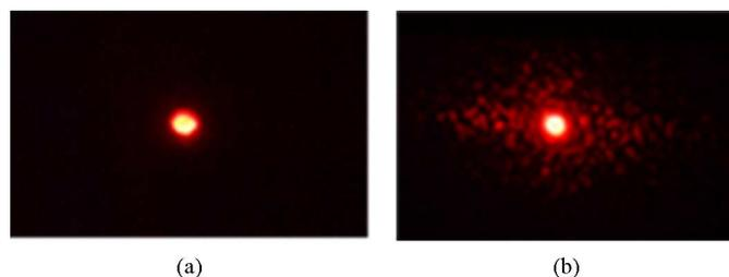
Fig. 5. Diffraction spots when the intensity of recording beams is (a) below and (b) above the critical level, 176 mW/cm<sup>2</sup>.
