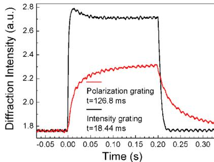
Fig. 8. Comparison of diffraction intensity and response time for intensity and polarization holographies with 488 nm laser,  $I_1 = 115 \text{ mW/cm}^2$ ,  $I_2 = 106 \text{ mW/cm}^2$ ,  $\theta = 21.7^\circ$ .
