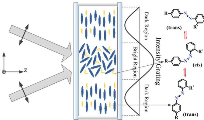
Fig. 1. Photorefractive mechanism of the azo-dye-doped LC.
