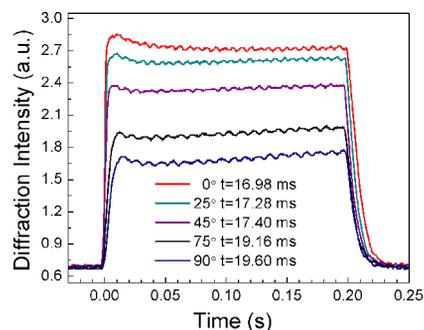
Fig. 6. First-order diffraction intensity and response time as a function of the angle between the recording light polarization direction and the director axis of liquid crystal  $I_1 = I_2 = 159$  mW/cm<sup>2</sup>,  $\theta = 21^\circ$ .
