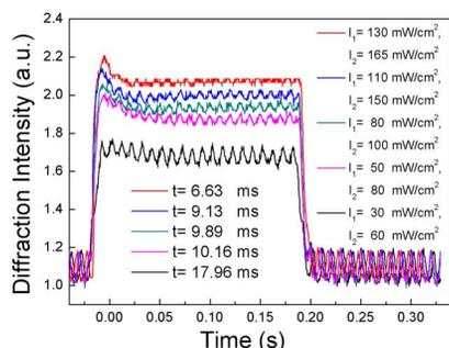
Fig. 4. Measured response time with respect to different combinations of recording intensities.
