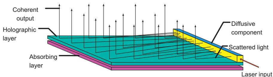
Fig. 2. Schematic system setup of the proposed coherent backlight system.
