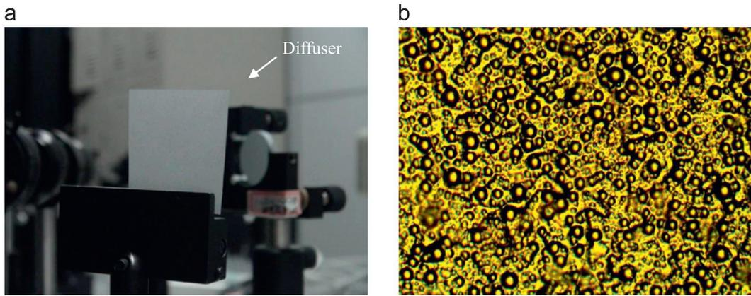
Fig. 3. (a) A diffuser from LCD backlight unit and (b) diffuser under microscope (100 ×) showing randomly structured surface.
