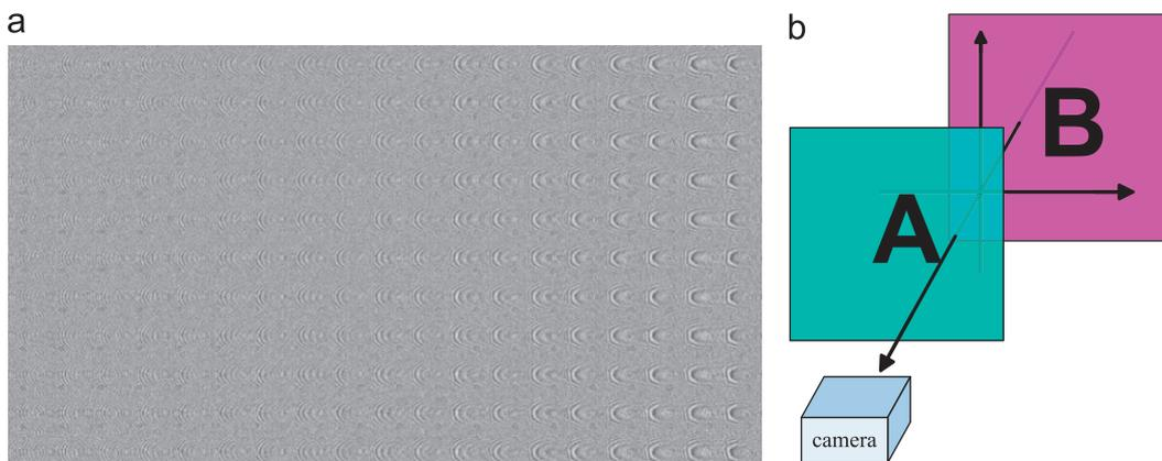
Fig. 6. (a) Computer generated hologram loaded on the SLM and (b) schematic diagram of the constructed 3D image in space with respect to the camera.
