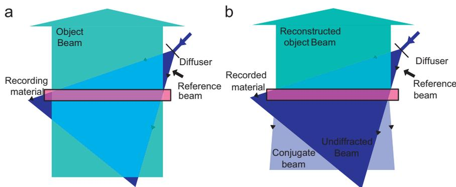
Fig. 1. Reflection hologram formation (a) and reconstruction (b) with scattered reference beam.
