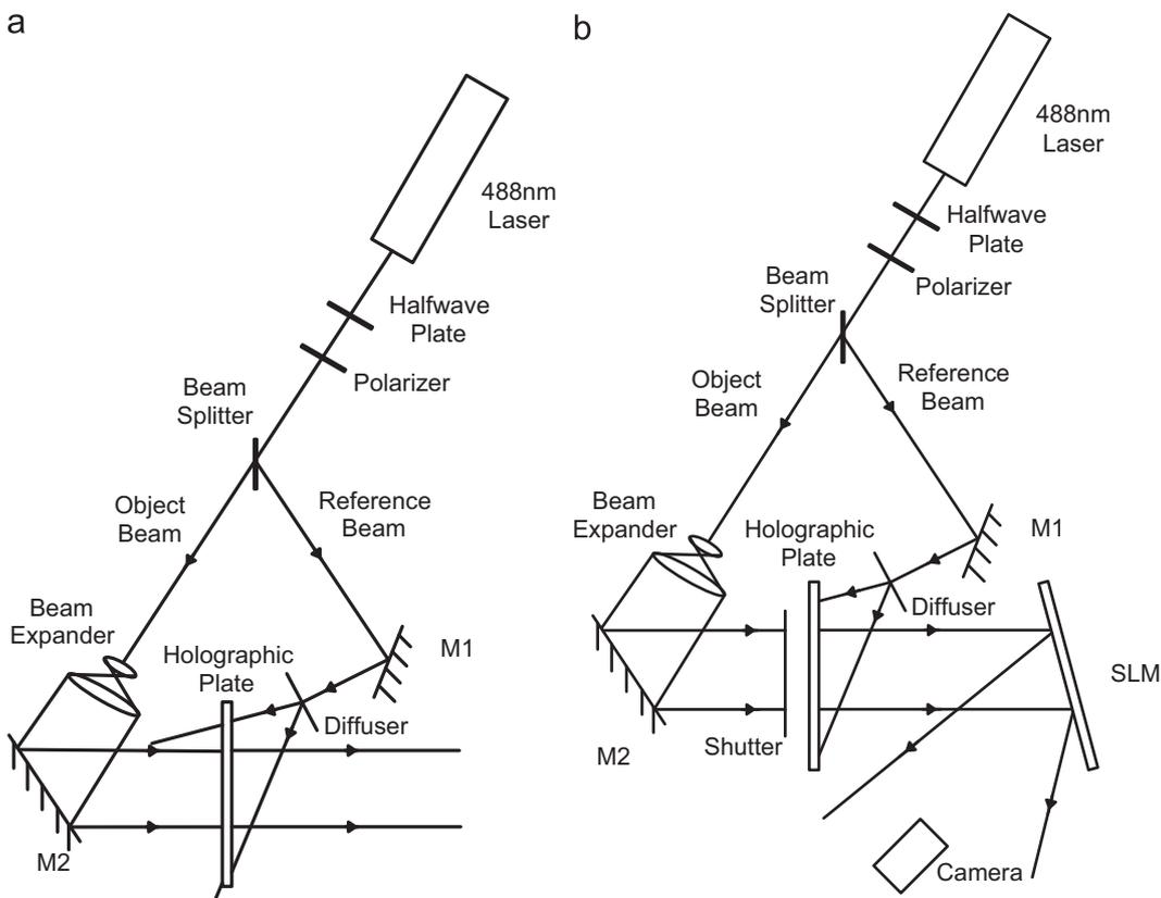
Fig. 4. Experimental setup for (a) hologram recording and (b) plane wave reconstruction.
