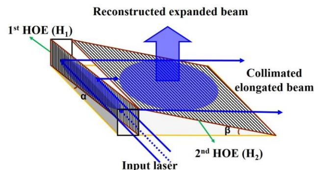
Fig. 1. Schematic drawing of the edge-lit coherent backlight.
