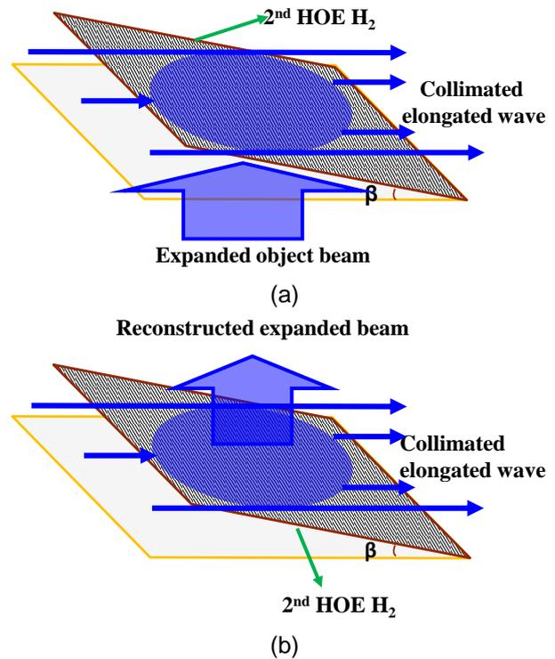
Fig. 4. Optical setup for H<sub>2</sub> during (a) recording and (b) reconstruction.
