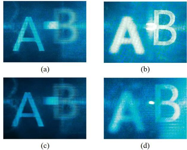
Fig. 6. Reconstructed holographic images by using the conventional beam expander when focusing on (a) 'A' or (b) 'B'; and by using the proposed edge-lit backlight when focusing on (c) 'A' or (d) 'B'.
