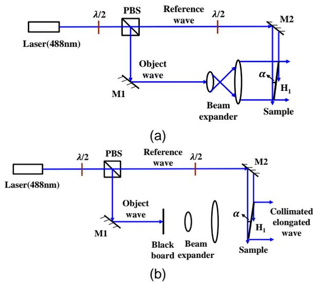
Fig. 2. Optical setups for H<sub>1</sub> during (a) recording and (b) reconstruction.
