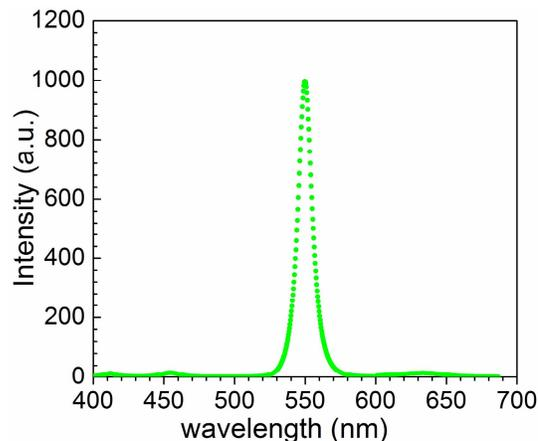
**Figure 4.** Spectrum of the emerging light from the device when  $n_{LC}=1.65$ .
