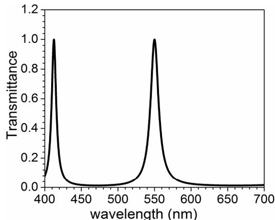
**Figure 3.** Spectrum of the blue phase LC FP filter when  $n_{LC}=1.65$ .
