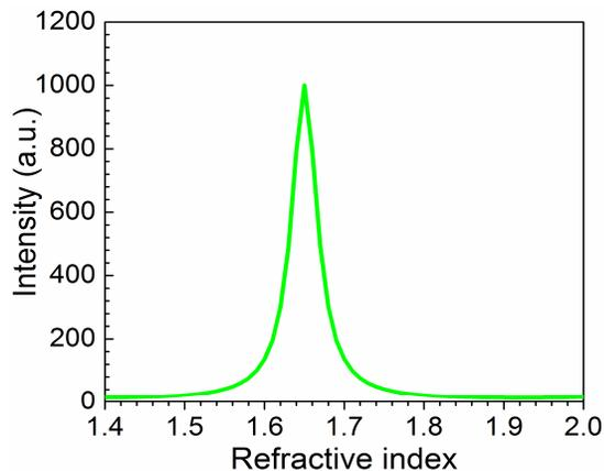
**Figure 5.** Intensity modulation through the variation of LC's refractive index.
