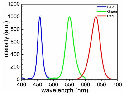
Figure 2. RGB spectra of quantum-dot backlight.
