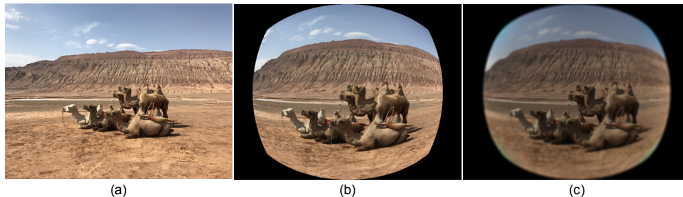
Fig. 11. (a) Original (photographer: C. P. Chen, location: Flaming Mountains, Turpan, China), (b) real, and (c) virtual images. By comparing the original and simulated images, it can be seen that the real image is inherently distorted at large field angles, while the virtual image turns out to be more blurred and more pronounced in the chromatic aberration.
