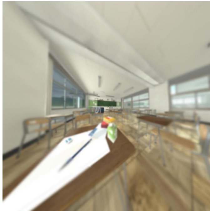
Fig. 5. Image with four regions being blurred with 1 \times 1 , 3 \times 3 , 5 \times 5 , and 9 \times 9 convolution kernels, respectively. The kernel size shall be inversely proportional to the ganglion density.
