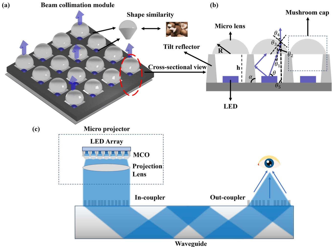
Fig. 1. (a) Schematic of the collimated LED array encapsulated with the MCO. (b) Cross-sectional view and the typical optical path of the LED array. (c) Schematic diagram of the working principle of an optical waveguide based near-eye display engine.
