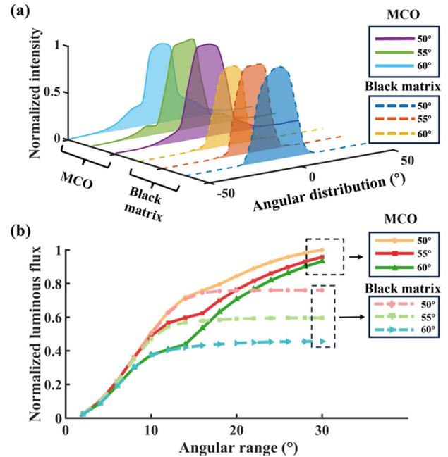
Fig. 6. (a) Comparison of the light intensity patterns between three different heights of MCO and the traditional black matrix. (b) Comparison of the light flux within the range between three different heights of MCO and the traditional black matrix.
