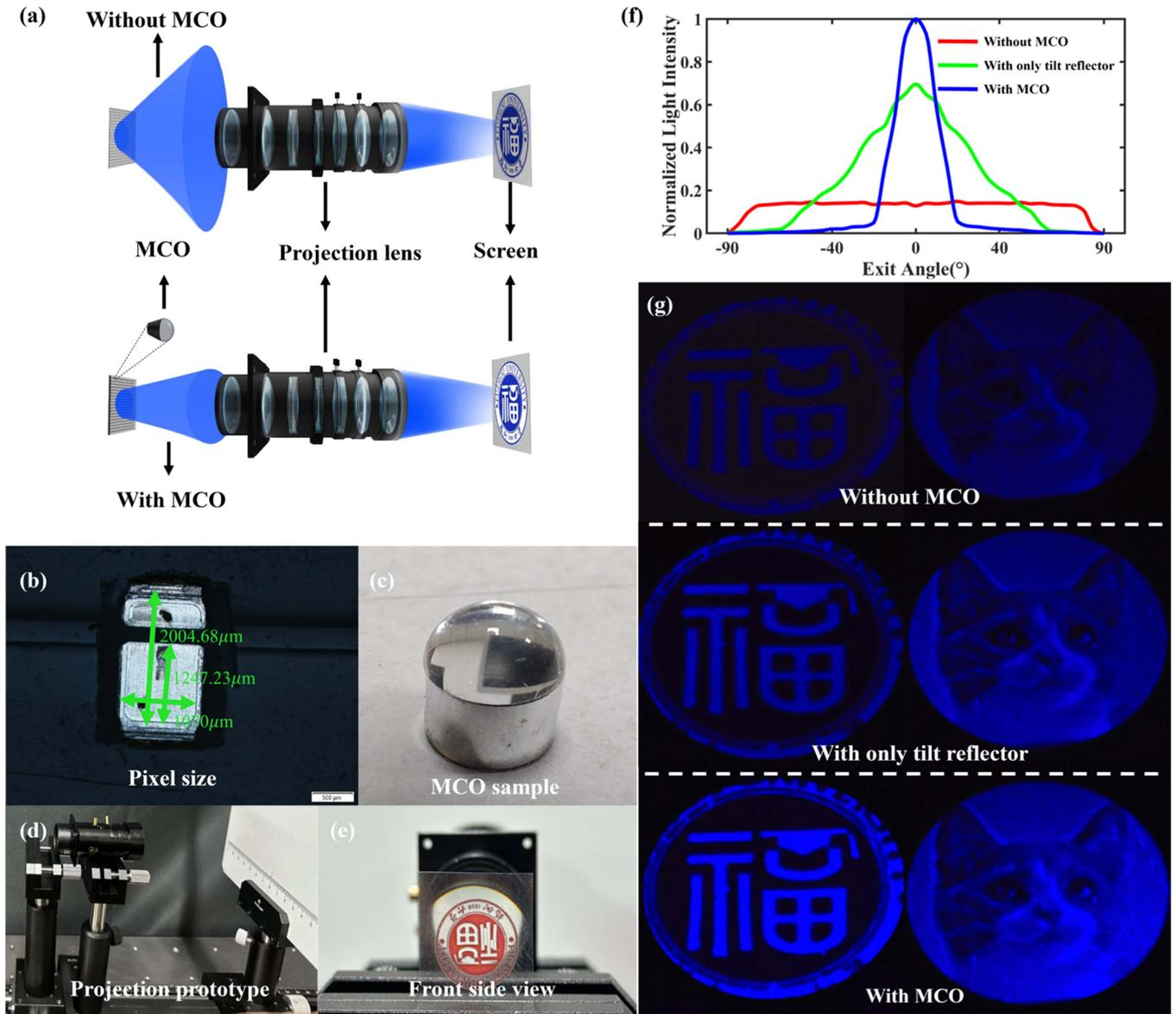
Fig. 7. (a) Schematic of the LED array projection engine with and without the MCO. (b) The LED light source used. (c) The fabricated MCO device. (d) Layout of projector prototype. (e) Front-side view of the projector. (f) The measured intensity distribution. (g) Actual projection effects of an untreated LED light source, tilt reflectors only, and MCO device.
