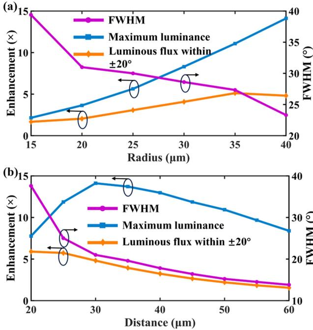
Fig. 2. Maximum light intensity, FWHM, and light flux within  $\pm 20^\circ$  corresponding to different micro-lens radius at the same placement height. (b) Maximum light intensity, FWHM, and light flux within  $\pm 20^\circ$  corresponding to different micro-lens placement heights at the same micro-lens radius.
