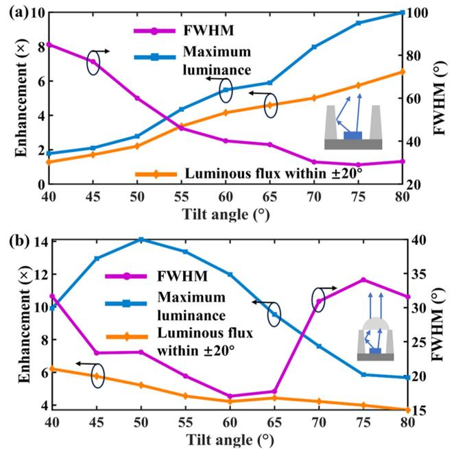
Fig. 3. (a) Maximum light intensity, FWHM, and light flux within  $\pm 20^\circ$  corresponding to different tilt angles of the tilt reflector for the same aperture size. (b) Influence of different tilt angles of the tilt reflector on the collimation performance of MCO.
